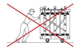
If a crane is not available when unloading the transformer from the vehicle, it is possible to unload the transformer with a forklift. The forks of the forklift truck, equipped with anti-slip guards, are inserted from the outside of the undercarriage beams. Special care must be taken not to damage the HV or LV outlets during this manipulation.
