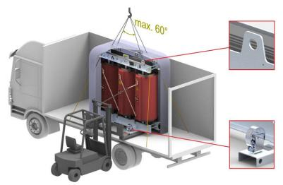
If the transformer is going to be transported by a forklift truck, it is recommended, after dismounting wooden prism, to place the transformer on these wooden prisms and then insert the forks into the undercarriage beams. If the transformer will continue to be transported on wheels, the wheels will be mounted on the undercarriage, after dismounting the wooden transport prisms.
