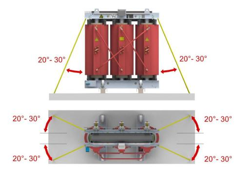
Even if there is no risk of the load slipping or overturning, it is recommended to take measures to prevent the unlocked load from moving freely due to vibration. The security measure must at least secure of withstand:
