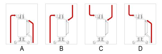
Depending on the customer's requirements, side LV terminals on the right or left side of the transformer can also be made.
