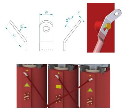
The termination of the LV terminals of the transformer is as follows:
